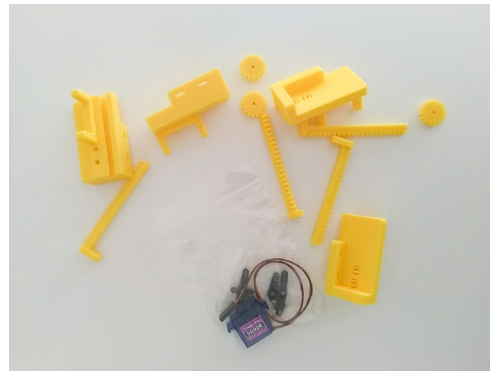
Figure 12. 3D-printed servo attachments
